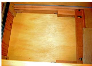
As a special feature, he designed the cabinet with hidden storage spaces under the bottom drawer, accessible after removing the drawer and the underlying panels. Except for the finger holes in the center divider, there is no visible evidence that there is any hidden space underneath the drawers. Clever idea, **Dan!**
